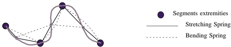
FIGURE 1. Spring distribution over a spline
